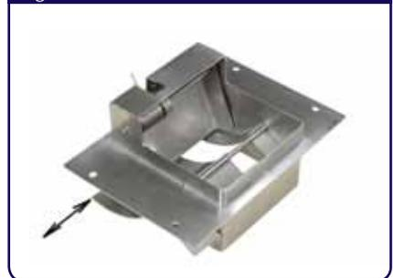
During commissioning (or for long-term production capacity change), the air flow through each STAFF can be adjusted without any spare parts by only side-sliding the flap and hereby changing the orifice area.
